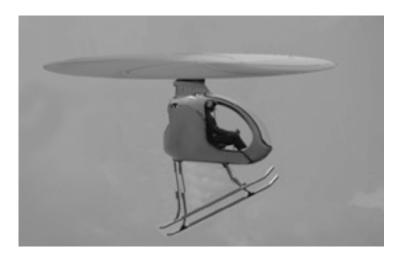
disc rotated overhead at more than six thousand rpm, several times faster than was possible with traditional blades. A series of thin slits scooped air in from the top, compressed it centrifugally inside and shot it out the bottom of the new rotor, providing lift. Shaped like a popular flying disc toy, the large disc incorporated an internal flywheel of identical weight that rotated counter to the main disc. This provided neutral rotational torque.
